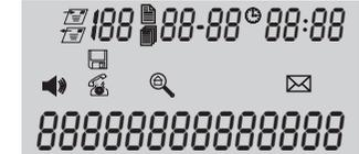
In standby mode, the LCD will show the handset number, date and real time.
