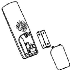
Insert two pieces Rechargeable AAA batteries in the compartment, ensuring correct polarity and close the compartment
