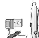
1. Connect the small plug of the power adapter to the power connector on the baby unit and the other end of the adapter to the mains socket (230V/50Hz).
