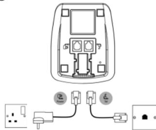
1. Plug the telephone line cord into the socket marked
