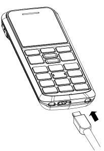
Connect the mobile telephone to the power pack. If the battery is completely discharged, it may take a few minutes before the telephone indicates that it is being charged and that it can be used for telephony. The telephone will indicate when the charging process has been completed.
