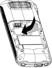
4. Insert the battery again and finally slide the cover back onto the case.
