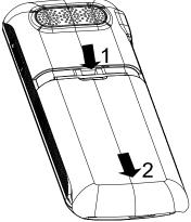
2. Take out the battery; remember beforehand the position of the battery in the mobile telephone with the contacts at top left.
