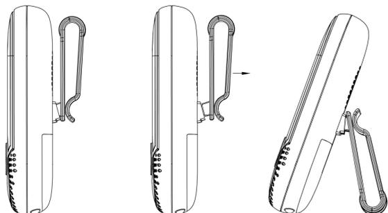
1. On normal state, the belt clip can be hanged on the belt directly.
