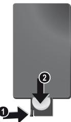
2 Insert the new batteries into the battery compartment with the positive and negative poles as shown on the back of the remote control. Make sure the polarities(+ and -) are aligned correctly.
