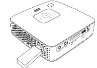
1 Connect the USB storage medium directly to the USB socket on the left side of the device.
